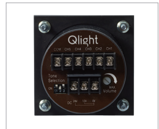
Terminal block for power and sound (back side, SPK)
